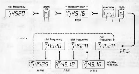
(Example for dual watch when there are memories in A-M1, A-M4 and A-M6.)
