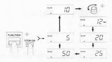
After setting channel step, depress # BZ S.C button to set previous mode.
