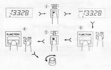
2 Switching semi-duplex and full-duplex It is initially set to full-duplex mode
