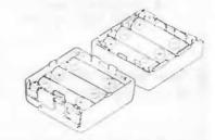
Install battery case into C500
