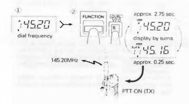
Note: If no memory is in "A-M1" or "B-M1", depressing D/ DUAL VFO button results in disablement with short beep.
